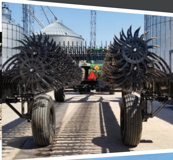
Yetter 3600 Pull-Type Rotary Hoes fold for narrow transport width of 11.5'.
