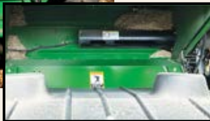
A tailboard, with the Tailboard Trash Blower Tube, after a full season of harvesting soybeans.
