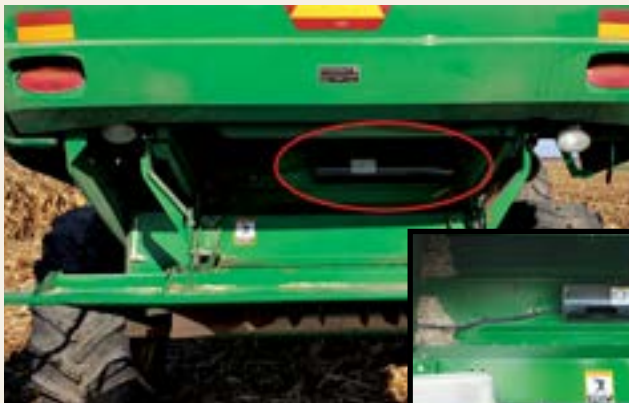
A tailboard, with the Tailboard Trash Blower Tube, after a full season of harvesting soybeans.
